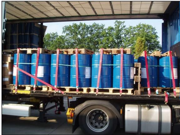
Example of good load securing with perforated metal profile:
