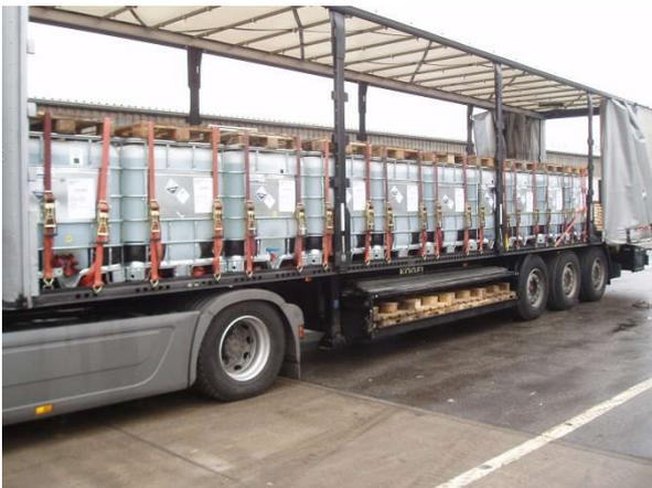
Example of good load securing with sufficient amount of pallets:
