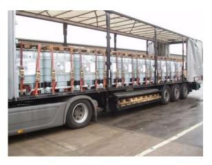
Example of good load securing with sufficient amount of pallets:
